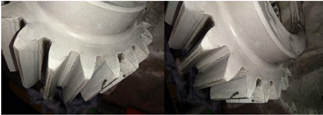
Failed replacement pinions
