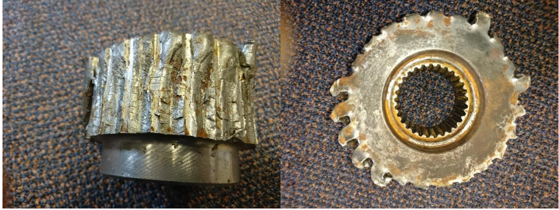
Failed original pinions
