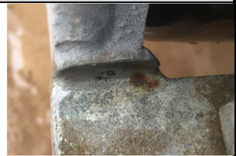
Crack Developing in Caster
